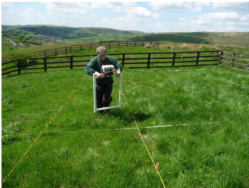
John Pitman from Tameside Archaeological Society undertaking the resistivity survey
