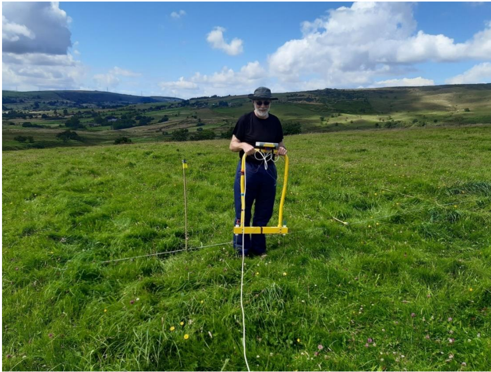
Figure 16 – Earth resistance survey equipment
