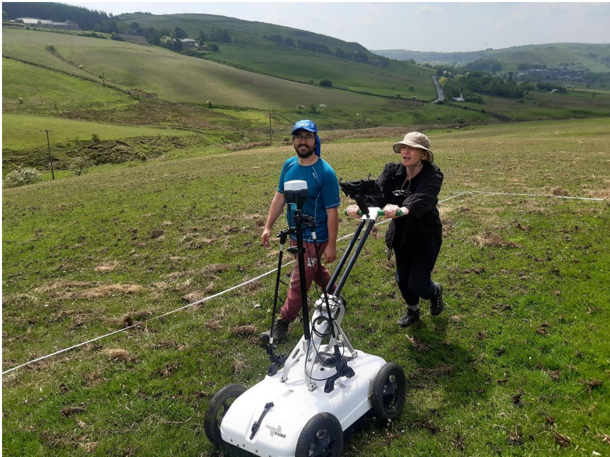
Figure 19 - Collecting GPR data on 500mm grid
