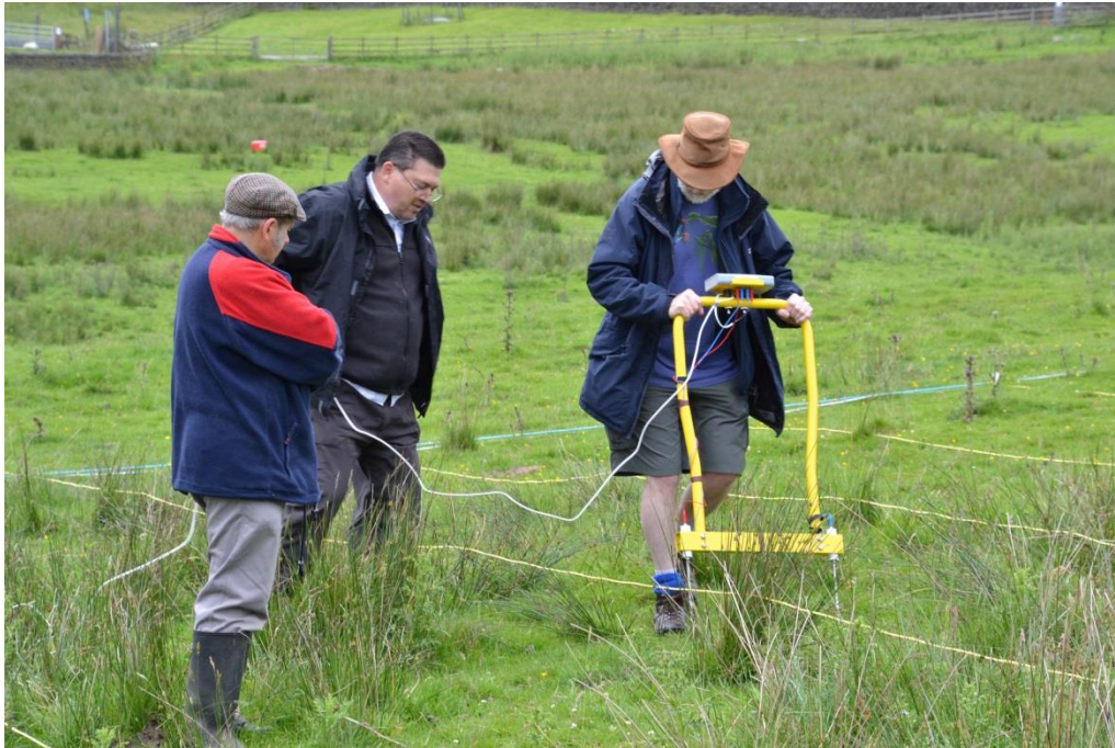
John Pitman, Terence Andrews and Phil Barrett use the Friends' recently acquired Frobisher Resistivity Meter.
